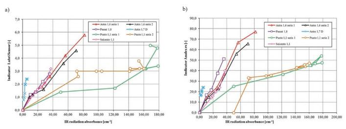
Fig. 8. Variation in infrared absorbance IR compared to the total base number measured by application of: a) Lubri Sensor b) Analexrs
